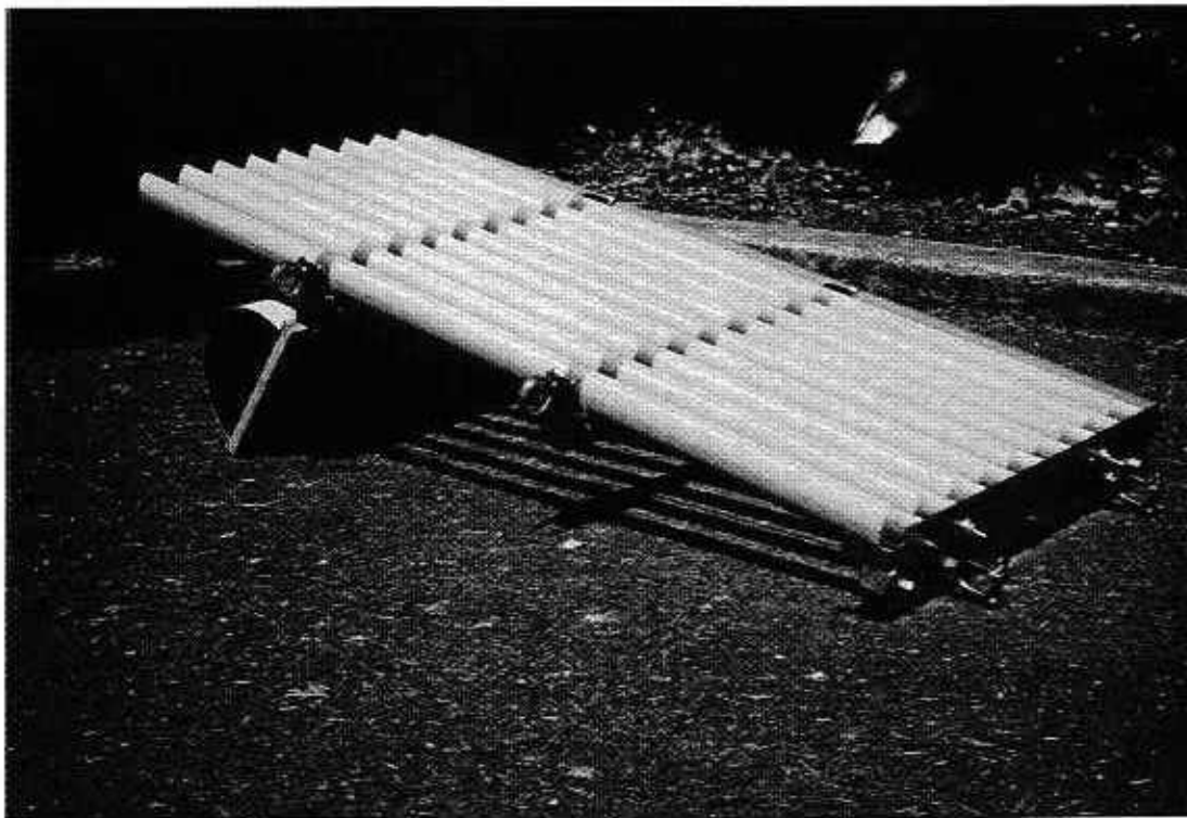
Appendix Figure A-9. Floating weir panel showing resistant board with extra flotation and attachment clamps (right side of photograph).
