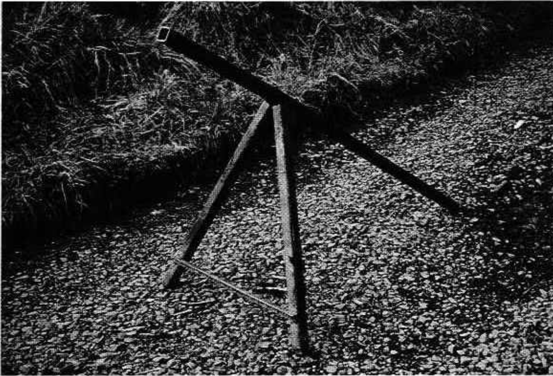
Appendix Figure A-2. Metal tripod with adjustable rear legs and metal front leg used with vertical picket weirs in the Siuslaw River, Oregon, 1995.
