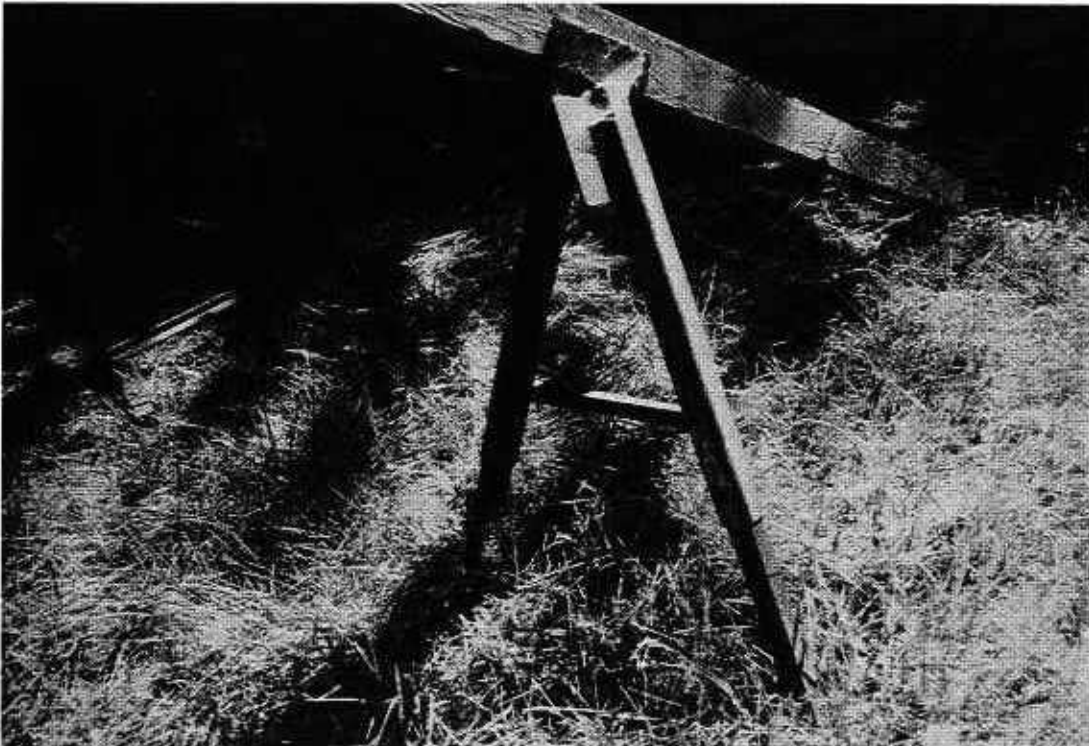
Appendix Figure A-1. Metal tripod with adjustable rear legs and wood front leg used with vertical picket weirs in the Siuslaw River, Oregon, 1993.
