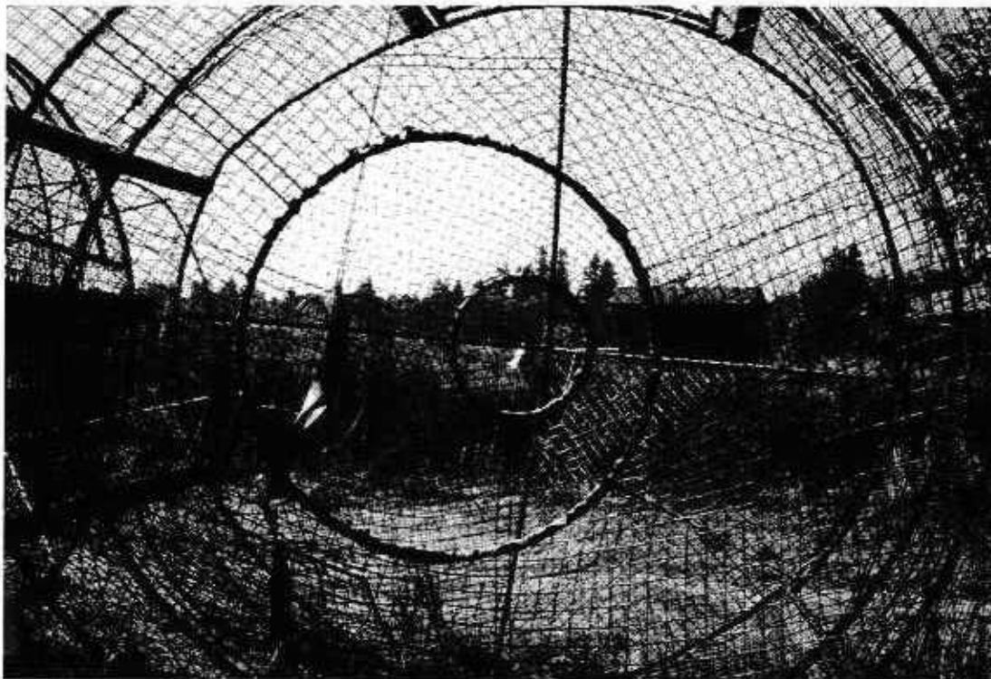
Figure 9. Downstream (larger) and upstream (smaller) fykes inside a hoop trap used to capture adult coho salmon in the Chehalis River, Washington.
